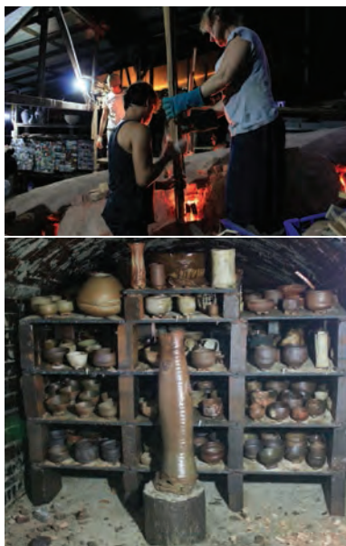
Top: Gently loading wood into stoke holes Above: The kiln open and photographed before unpacking
